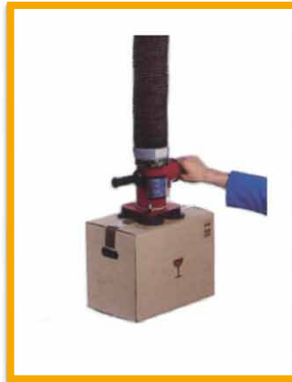
Cardboard sucker with bellows 30 kg load
